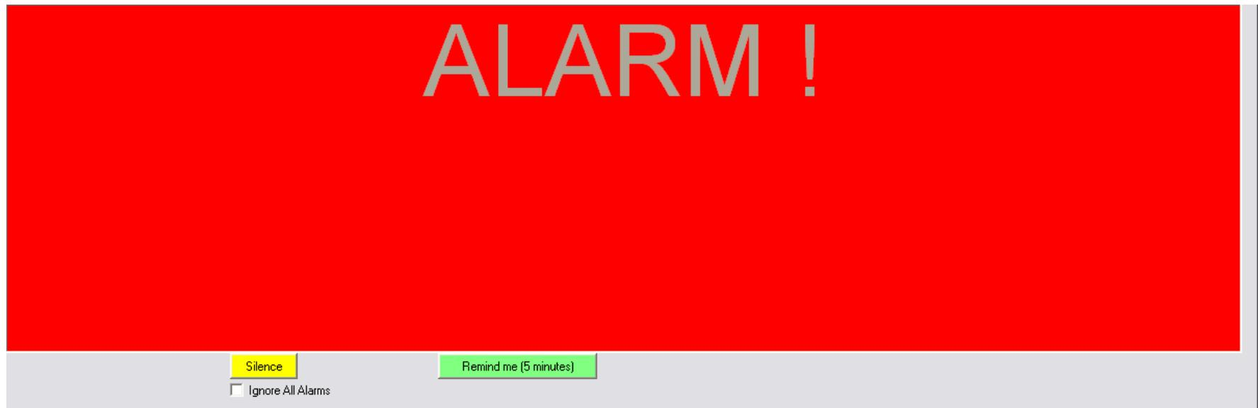
The on screen alarm alerts the user to any system malfunction or, optionally, the alarm will display if bale weight or %AD exceeds the defined limits.
